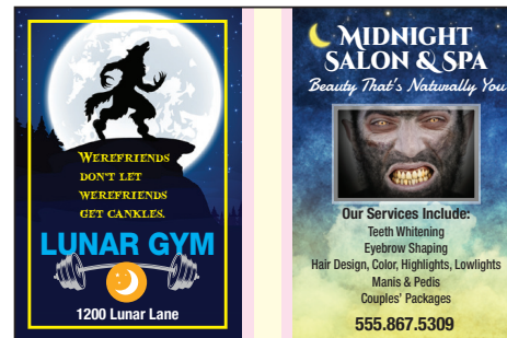
Figure 2. Perfect bound cover: inside. The yellow area represents the spine. The pink areas represent the hinges where the cover will glue to the first and last interior pages. The yellow area must be free of ink. Allow a larger margin on the spine side (pink areas) of the inside covers to prevent text from getting glued inside the hinges.
