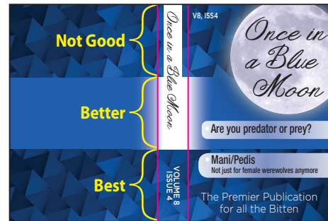
Figure 1. Perfect bound cover: outside. This is one example of color transitions across the spine. The general idea is to avoid hard color changes if you're concerned about the little bit of rolling that can happen during application. The pink lines represent the hinge score. You may want to avoid positioning text where the scores will run.
